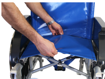
Figure 3, Folding the wheelchair
