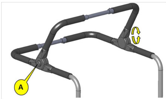
Figure 43: Angle adjustment of the pushhandle
