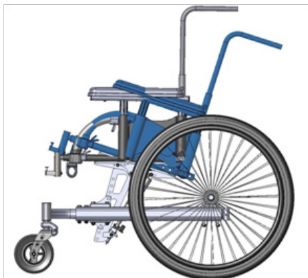
Figure 8: Tilt limitation on 4 wheels configuration with extension plates.
