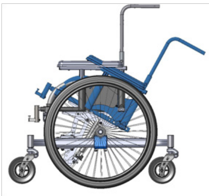
Figure 9: Tilt limitation mid wheel configuration with extension plates
