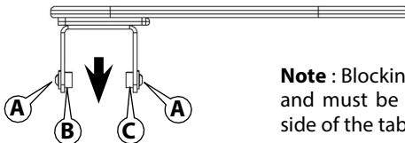
**Note :** Blocking bar **B** is thicker than **C** and must be placed on the opposite side of the table, as illustrated.
