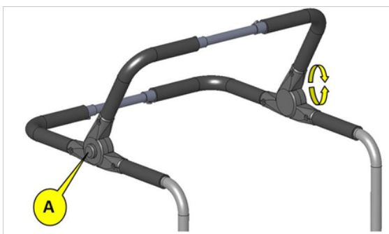
Figure 43: Angle adjustment of the pushhandle
