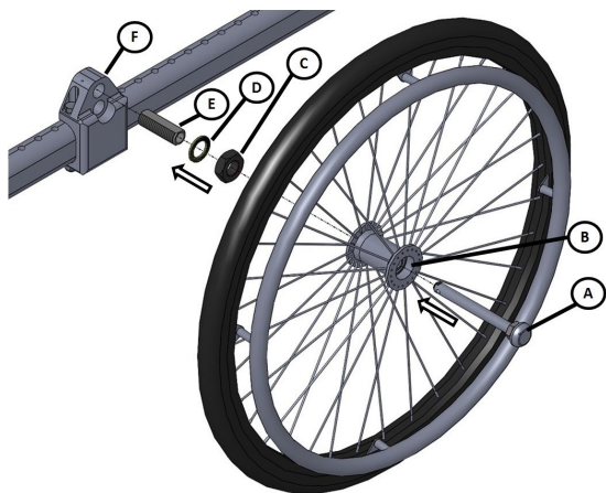
Figure 14 : Rear Wheel Installation
