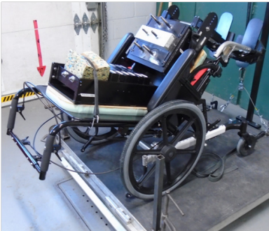
Figure 5: Rearward stability test with a reclining backrest on the NEOX tilt in space.
